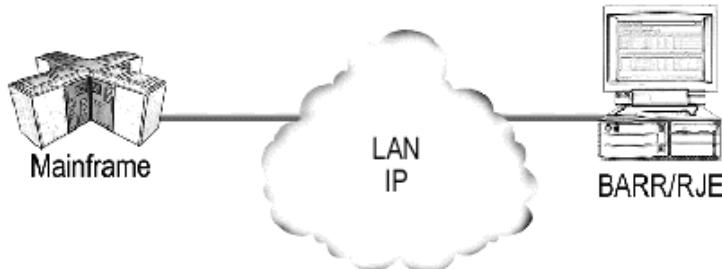
HPR/IP connections attach to the mainframe using IP.
